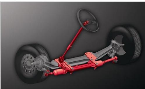
Freightliner's industry-first rack and pinion steering system , available with spring or front air suspensions, is responsive and provides tight control.
