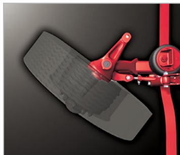
The wheel wells and chassis geometry allow a tight wheel cut of up to 50 degrees for greater maneuverability.
