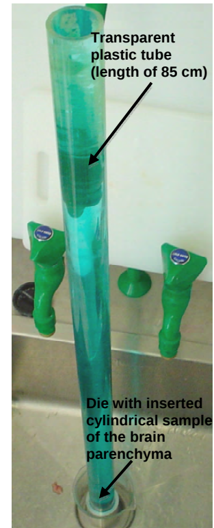
Fig. 1 Experimental set-up with 85 cm CSF column applying pressure on the cylindrical brain sample inserted into the die.
