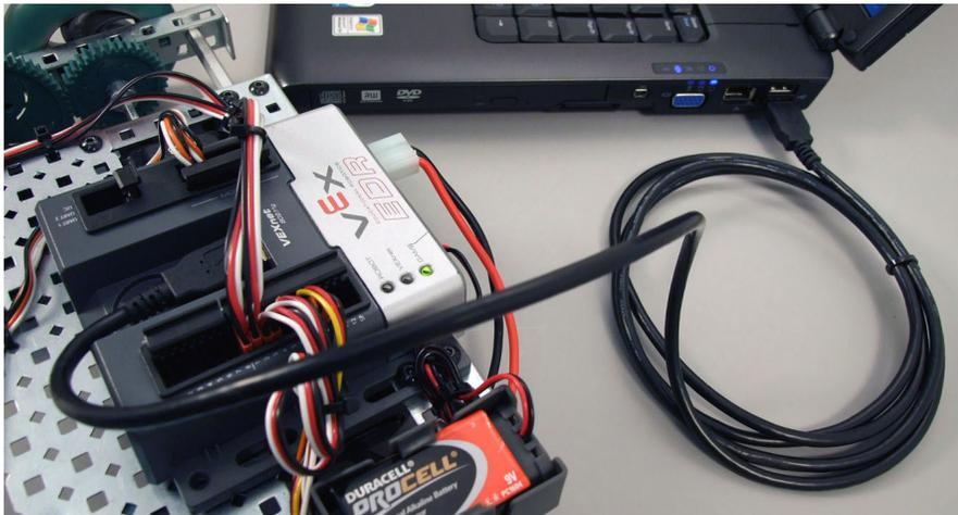
2. Open *ROBOTC for Cortex and PIC*. ROBOTC will automatically recognize which USB port your robot is connected to.
