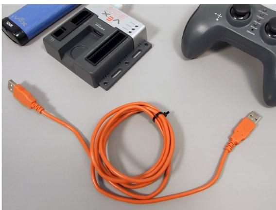
6. Insert VEXnet USB Keys into both the VEXnet Joystick and Cortex.
