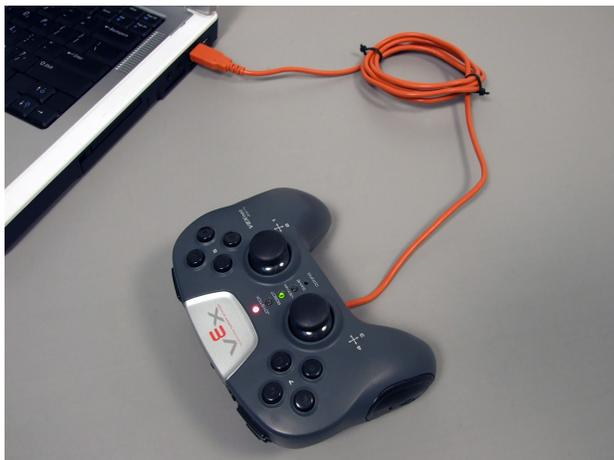
**2a. Connect the VEXnet Joystick**
