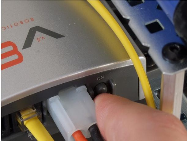
4. Turn on the Radio Control Transmitter and observe the robot. You will need to use the transmitter joysticks and buttons to test the user control period.
