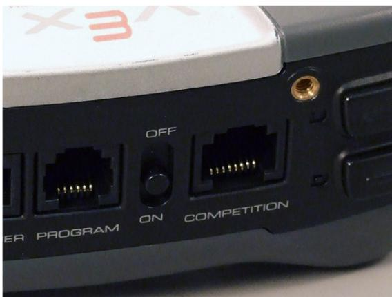
7b. Turn the VEXnet Joystick ON
