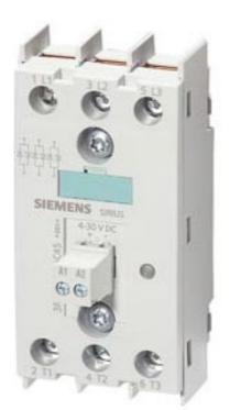
SOLID-STATE RELAY 3-PHASE 3RF2 30 A 40 DEG. C 48-600 V / 110 V AC 3-PHASE CONTROLLED SCREW TERMINAL BLOCKING VOLTAGE 1200 V
