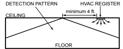
If the sensor's location gives it a view of other rooms or hallways, lights will be turned on when movement is detected in these adjacent areas. The sensor's detection zone may be restricted by masking a portion of the lens; or move sensor to eliminate detection through doorway.
