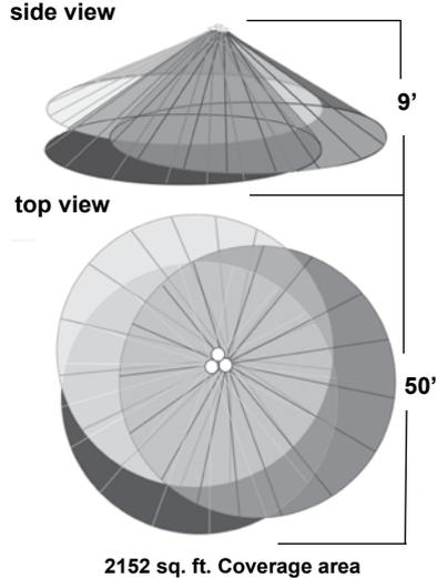
The LOS 2500 has 3 separate 360° detectors. Triple overlapping coverage provides super sensitivity and reliability.
