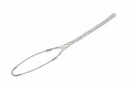
FC062U: Standard Duty, Closed Mesh, Single-Eye Grip, Cable Diameter 0.62 - 0.74 inches, Bale Length 8-in, Mesh Length 11-in, Break Strength 960 lbs.
