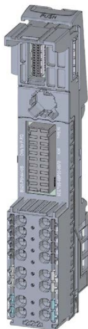
Figure 4-27 BU type F0, dark-colored version, with AUX terminals, supply over supply terminals
