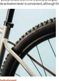
The skinny hydroformed seatstays (above) provide a degree of compliance, while the flared head tube (right) is designed for stiffness
