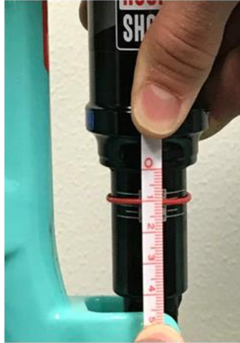
Measuring the SAG in mm- Step 2 [6]
