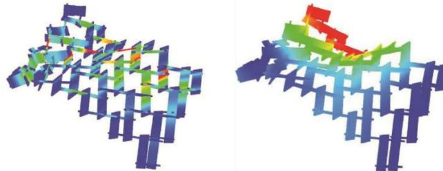
Figure 11: Bending moment and deflection visualization
