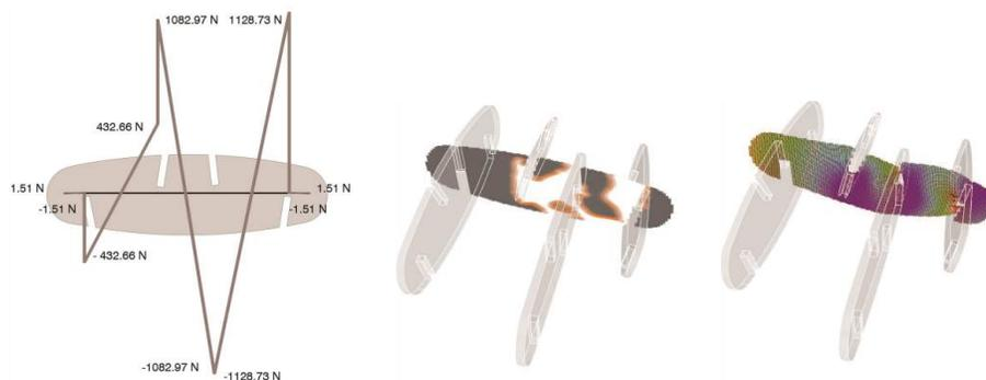
Figure 16. Tension forces extracted from the structural analysis, and stiffness and deflection visualizations
