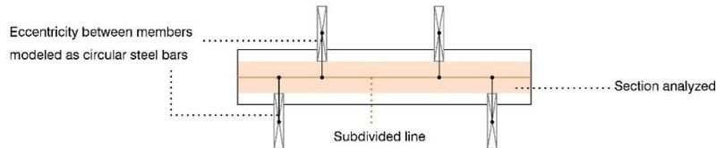
Figure 10: Structural model of planar reciprocal frame member
