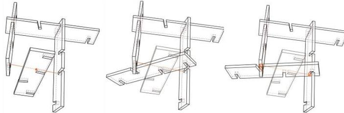
Figure 9: Rotation of member to check collisions
