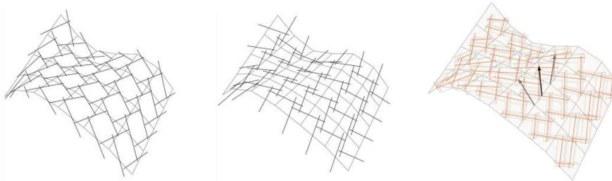
Figure 7: RF options by adjusting the angle (left and center) and panel orientation according to normal vectors (right)
