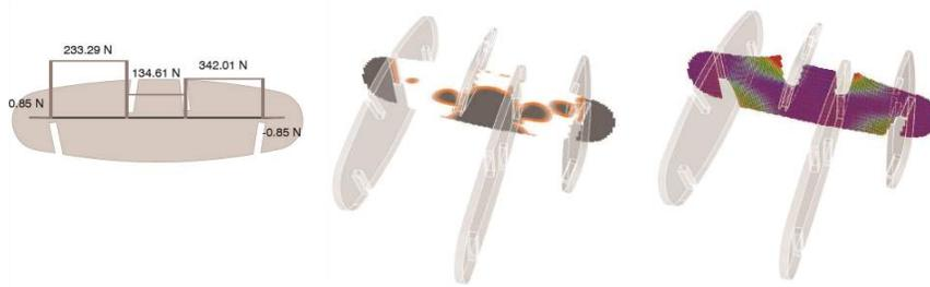
Figure 18. Axial forces extracted from the structural analysis, and stiffness and deflection visualizations
