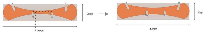
Figure 15. Minimum depth check and fix on a concave member
