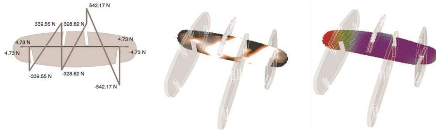
Figure 17. Torsion forces extracted from the structural analysis, and stiffness and deflection visualizations
