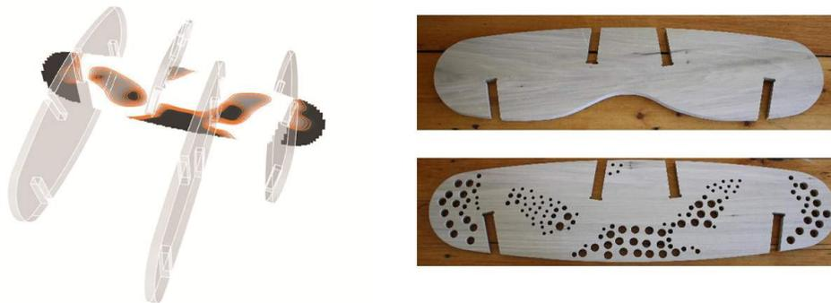
Figure 21. All load cases stiffness visualization and mass-customized boards
