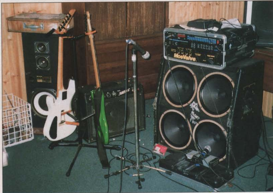
BOOGIE NIGHTS: The guitar was recorded using a Boogie 4x12 stereo box miked in front by a Shure SM58 and also with another mic in the back of the open cabinet.
