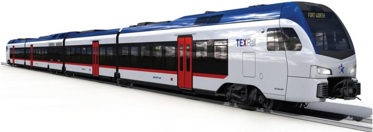
Self-propelled, diesel multiple unit trains have a role to play in HPR systems, particularly on important lighter-density routes that act as feeders to the heavily-travelled main trunk lines. These Swiss-designed cars are now being built in Utah for use on the TEX Rail service in the Dallas-Fort Worth area. Several other designs are now available for North American service.
