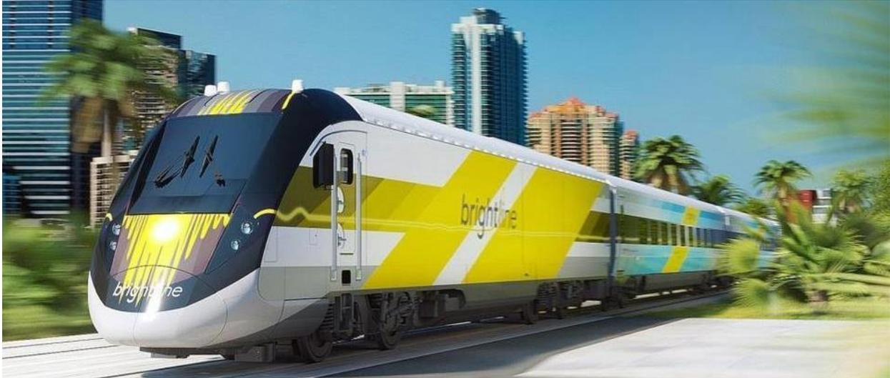
Based on highly successful locomotives and rolling stock in service in Europe, the single-level Siemens Brightliner trains have been built in California for the Miami-West Palm Beach-Orlando HPR service that will begin operation in late 2017.
