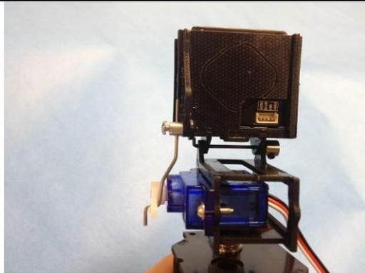
16. Place nylon spacer onto shaft followed by the tilt platform and star nut. Center the pan servo and place tilt platform pointed 180 degrees from the desired direction. Hold the bolt with a screwdriver (DO NOT APPLY FORCE AGAINST THE SERVO). Rotate the tilt platform, making sure the bolt is moving, until the bolt is tight and the platform is facing the proper direction.
