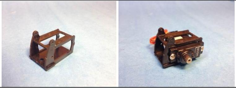
14. Align holes for camera housing and tilt base and insert "L" shaped wire. Use collet to secure as shown.
