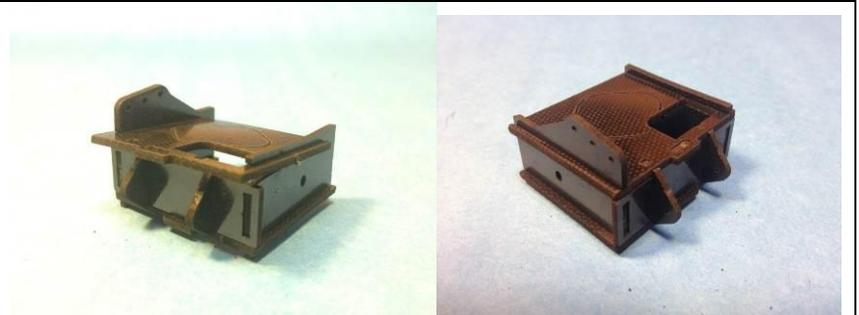
13. Assemble and glue tilt base as shown. Insert servo with gear output towards the hinge tabs.
