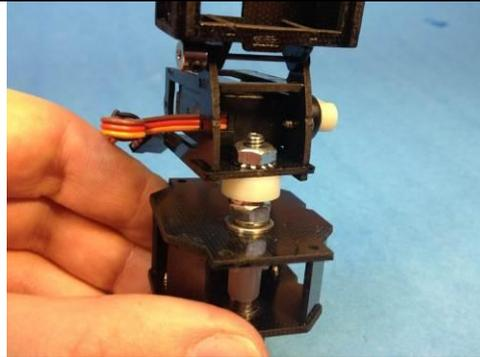
17. Place CCD camera into housing and secure with included fasteners. (Blue Loctite may be beneficial)
