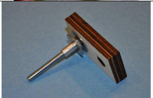
Test fit the spacers in the holes on the main body of the pan/tilt assembly. If they won't fit or if they don't spin freely, use a hobby knife to scrape a small amount of material from the holes on the top and bottom plates until the threaded spacer slides through without binding. Do not remove too much material or there will be excess slop in the pan assembly.
