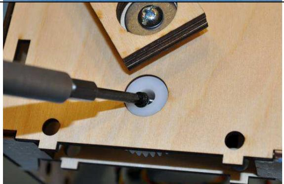
Add the two spacers to the front plate as shown. Glue in place.
