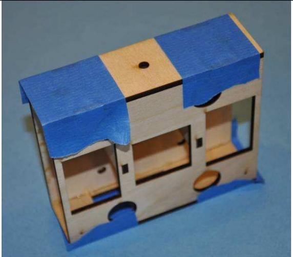
Mount the servo as shown, with the spline aligned to the middle of the side of the pan assembly.
