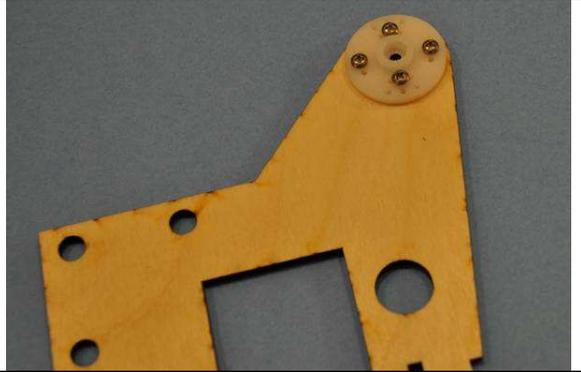
Install bottom platform to side support as shown.
