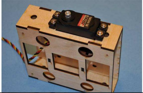
Insert the screw through the hole on the side plate and into the hole on the side of the antenna support. Note that extra room is left here to account for the use of servos that have different heights.
