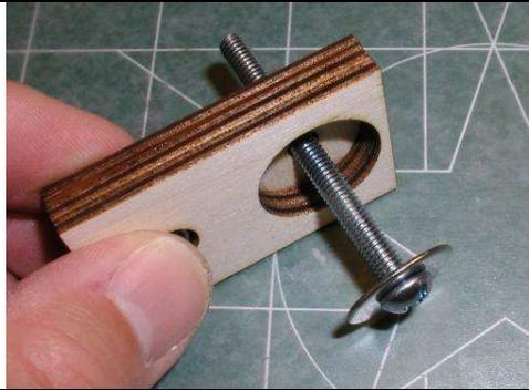
On the opposite side, add a washer and a nut. Tighten securely.
