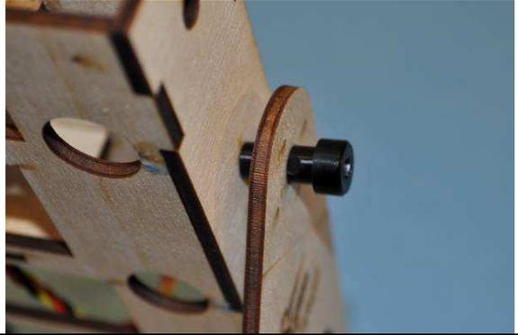
Add the nut to the inside and tighten securely. Add thread lock.
