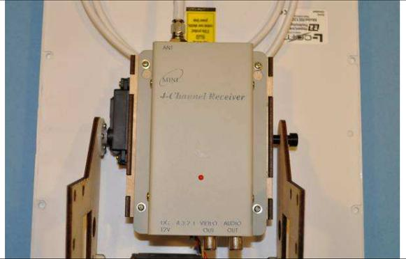
The Eagle Eyes unit is mounted to the side plate using adhesive Velcro and the Velcro strap. The adhesive Velcro can be placed in an "I" configuration with one longer strip up the middle and two shorter strips across the top and bottom.
