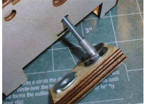
With the bolt partially inserted through the bottom hole, drop in the small gear in the orientation shown and slide the bolt through the gear. A set of needle nose pliers may be helpful in this step for holding the gear.
