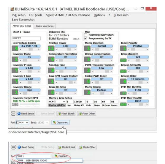
4. Connect ESC with suitable battery and click button "Sead Setup", then you can see the indication "ESC#1 setup read successfully"
