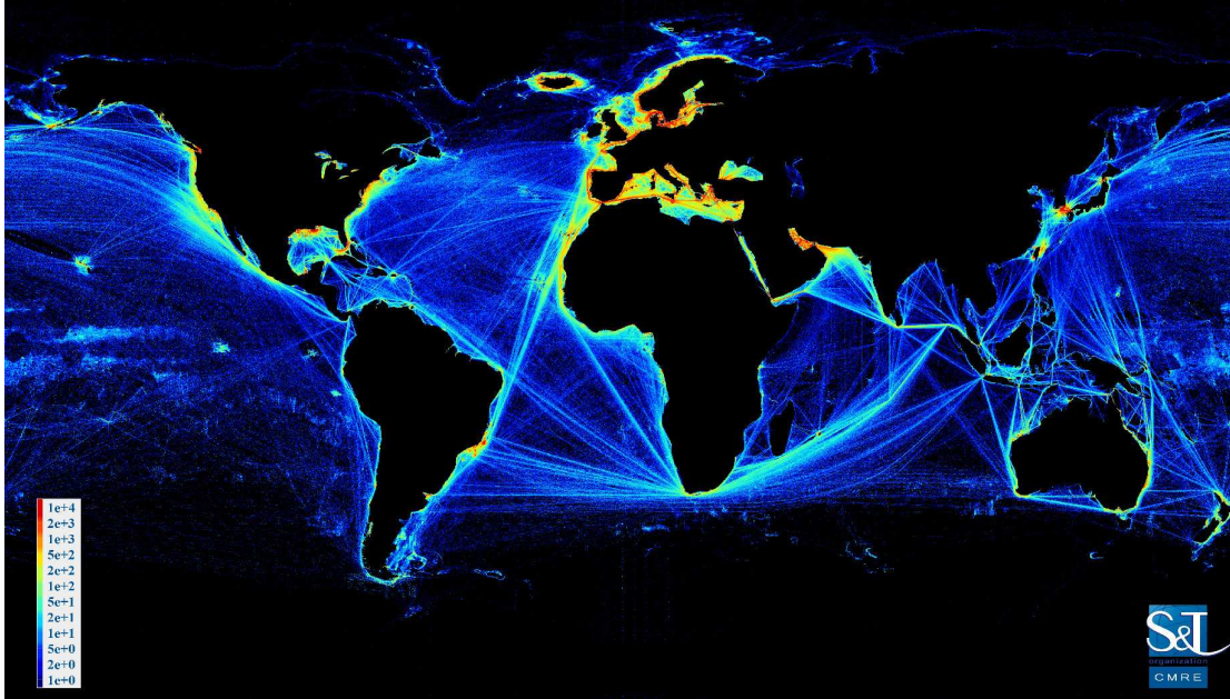
Fig. 1. Density of Automatic Identification System (AIS) messages collected from multiple AIS networks from April to September 2012. Each pixel covers a 4 nmi (one-fifteenth-degree) square on the ground and its color is (logarithmically) proportional to the number of ships whose reported position fall within its footprint.
