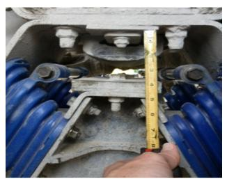
Above is a picture of ATRO load springs (LP50-24179) and OEM Auxiliary Spring which shows the auxiliary spring height is slightly over 2 1/4". The height of the spring should be 3 3/8". Per OEM specifications, the spring should be replaced when the spring height is less than 3". This auxiliary spring should be replaced.
