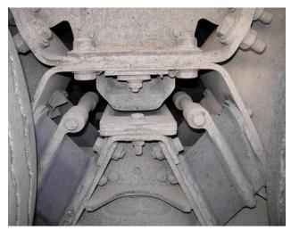
Above is a picture of slightly used ATRO load pads (LP50-24179) and ATRO auxiliary spring (LP50-24974). The gap between the spring and top shim plate appears to be good (less than 3/8"), however, the top shim plate is worn completely through. This forces the suspension to lower another 1/4" before the auxiliary contacts the second plate. This shim plate should be replaced.
