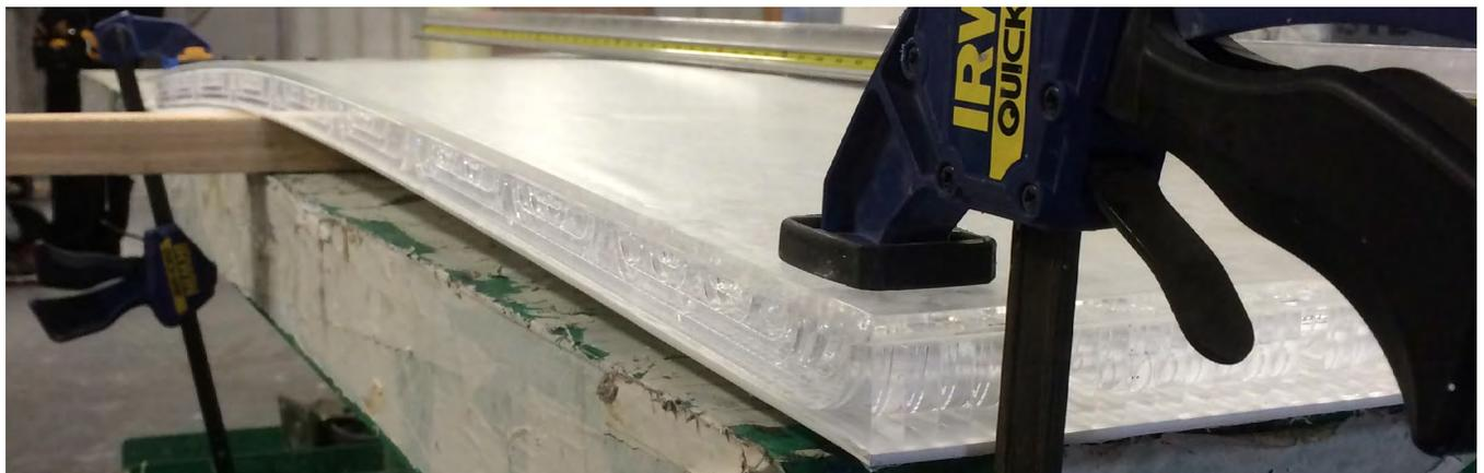
When uninstalled, it is not uncommon for panels to bend in response to changes in temperature and humidity. This is nothing to worry about however, because the proper attachment methods are stronger than the panel's need to bend and will flatten it out.
