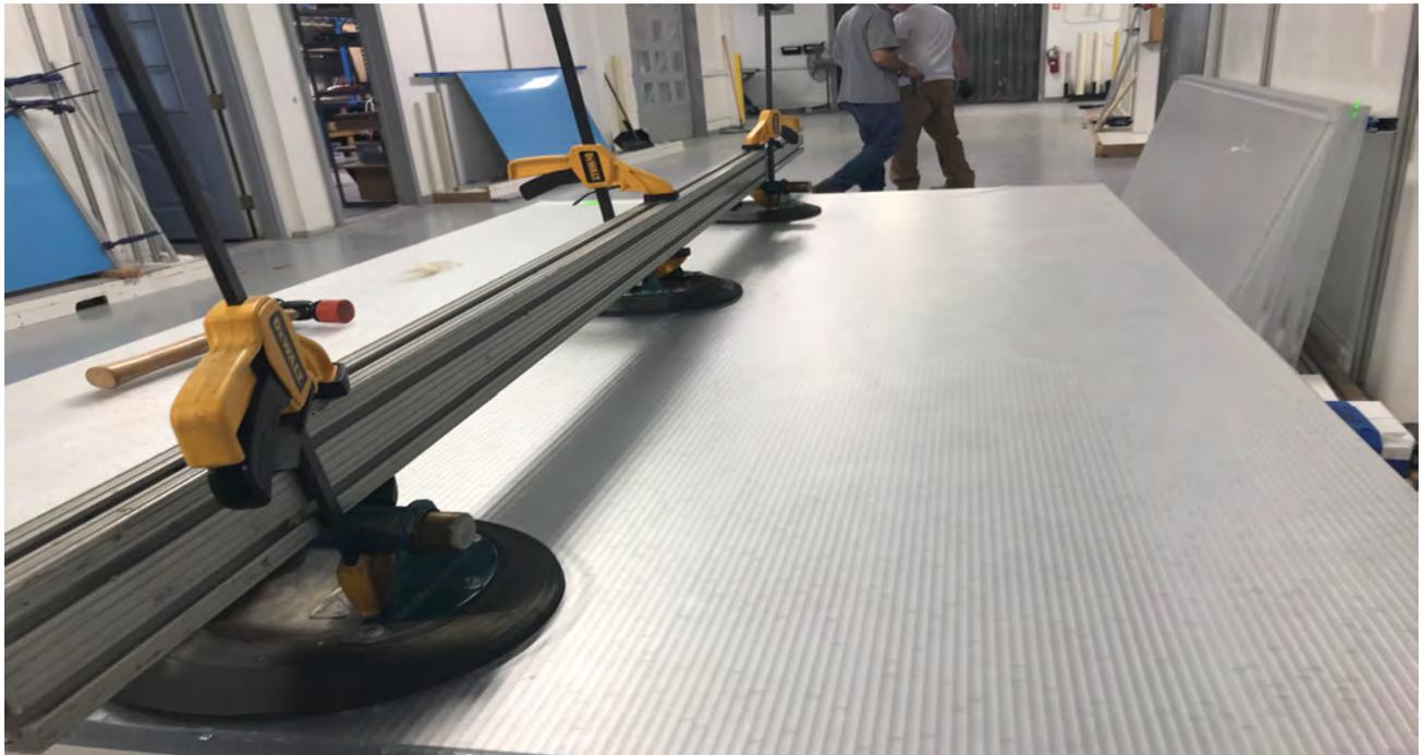
Suction cups combined with a rigid bar and clamps are used to lift and flatten panel that may be too heavy or awkward to be able to apply pressure where needed to engage the z-clips
