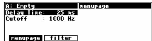
Also notice that because the second `knob` module “took over” the `filter` module's `frequency` control input, that parameter no longer appears on the `filter` module's menu page.
