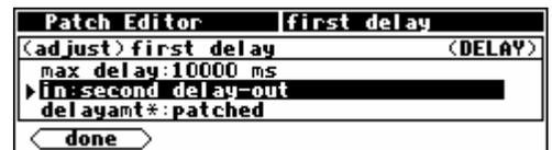
Returning to the basic Patch Editor area display (*by pressing the <done> SOFT KEY*), we can see that the second `delay` module's output is indeed connected to the first `delay` module's input.
