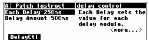
The menu page shown above is visible in the PARAMETER area. It is created with a *menupage* module, a knob module, a monitor module, and a *textblock* module (*we'll see how in a minute*).
