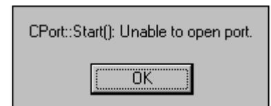
Vsigfile will itself hog the comms port. To “disconnect” Vsigfile from the comms port (so that you can use another device), choose Disconnect from the Midi menu, or use AutoDisconnect which will disconnect the comms port after it has not been used for a while.
