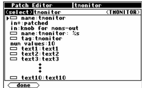
Both the textual monitor modules create displays that are half of a screen width and one line long.
