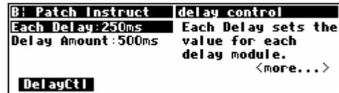
For the sake of demonstration, we'll use the **<connect>** SOFT KEY to rearrange the **delay (dly)** modules such that one is in "channel" 1 and the other is in "channel" 2, thus delaying each "channel" by up to 10 seconds (10,000mS). (*Hey! Ya gotta crawl before you can run, OK?*)
