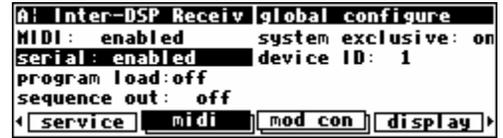
If you find that your PC is “unhappy” about the speed of transmission (as in “it’s too fast!”), lower the **sysex speed** parameter on the “second” **[midi]** menu page in the SETUP area. This will dumb down the Harmonizer’s transmission speed.
