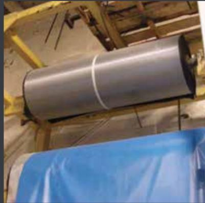
**Photo 1** CSPE resin headed into the #11 mixer.
