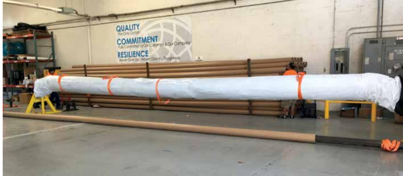
**PHOTO F** Finished panel, rolled up and packaged. 7,875 square feet per roll / 3,800 lbs. per roll.
