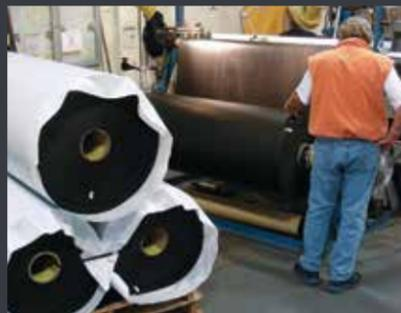
**Photo 5** Checking mill thickness at the inspection station.
