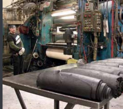
**Photo 2** CSPE on warm-up/breakdown mil prior to being fed into the calender.
