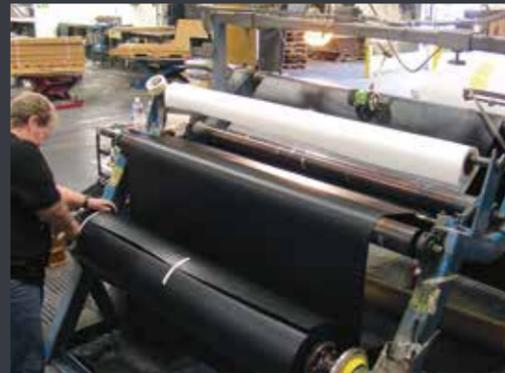
**Photo 4** CSPE material for Palos Verdes in inspection station with an ethylene propylene rubber (EPR) compound finish.
