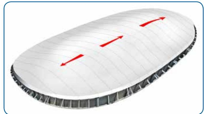
**CONSIDERATIONS:** Check weather conditions prior to starting your installation, do not try to deploy covers in windy conditions. During and after deployment, some type of ballast must be used to prevent wind from taking control of the cover material, aeration fans may also be utilized. Typically, sandbags are used for ground piles without aeration and should be placed as required to prevent damage to the cover during installation.
