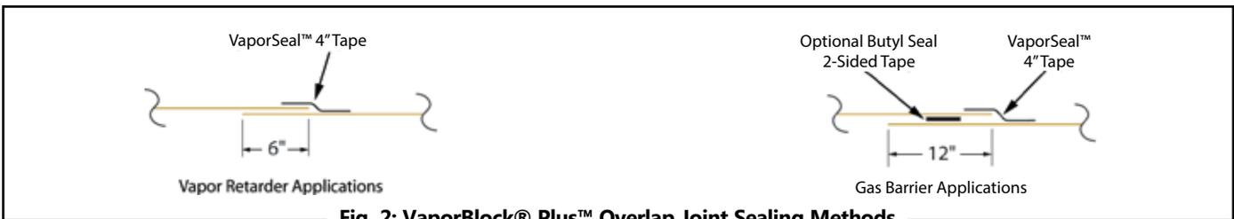
**Fig. 2: VaporBlock® Plus™ Overlap Joint Sealing Methods**
