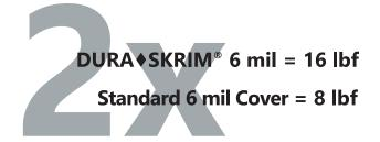
Puncture Strength Test - ASTM D4833 Competitor Covers based on average of four specimens, rounded for single value.
