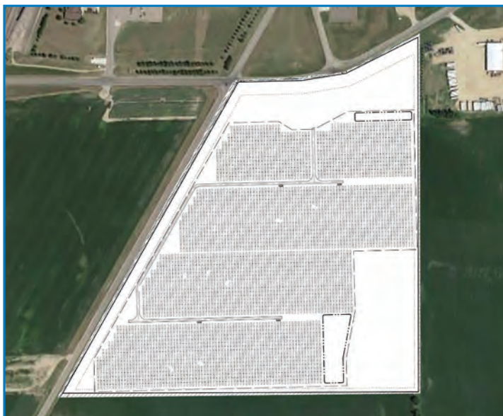
The Marshall Solar Plus project is projected to be a 10-MW capacity solar farm and 5-MW battery-storage facility located on a quadrangular-shaped property MRES owns on the northern outskirts of Marshall, Minnesota. The solar facility will cover approximately 55 acres and will feature single-axis solar panels that follow the sun from east to west. Note: This graphic is for illustrative purposes only.
