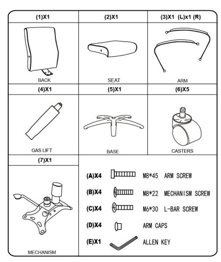
Insert and loosely tighten all screws. When assembly is completed, fully tighten all screws before using. This chair is only intended for sitting. Any other use will void the warranty.
