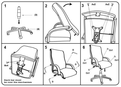
Note: Please tighten all arm screws using allen key before step 6
