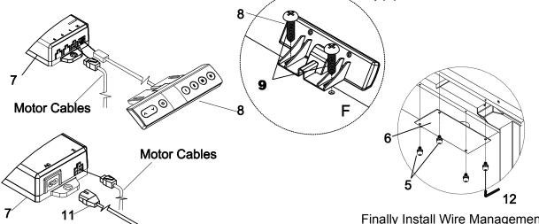
Finally Install Wire Management Tray (6) to Frame using Screws (5) and Wrench (12).
