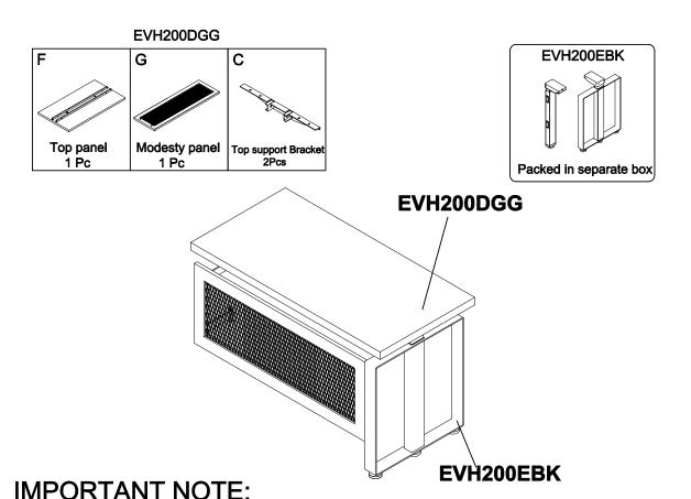
Place all wooden parts on a clean and smooth surface such as a rug or carpet to avoid the parts from being scratched Check that you have all parts and hardware.
