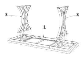
2 Thread one nut (B) through each end of the support rods (2) and add a washer (C). Place the support rods (2) between each side leg frame (3) and align them to the middle of the desk. Adjust each leg frame so that the holes align with the screw points on the bottom of the desk top.
