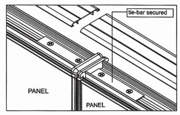
**Step 4**: Once all the 4 screws are secured then fix back the aluminium top cover by snap fit.
