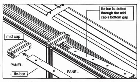
Step 2: Slot in the tie-bar through the bottom gap of the mid cap.
