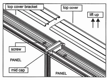
**Step 1**: Lift up the top cover and unscrew the 2 screws from the top cover bracket next to the mid cap.
