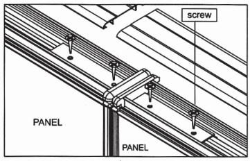
**Step 3 :** After the tie-bar is securely placed, please drill 4 holes through the top cover bracket to screw in or just use self drilling screw for securing the tie-bar.
