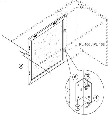
Attach L-Bracket #2 to Glass Modesty Panel (A) with hole marking (6 pcs in total) and to PL 466 / PL468 by using 12pcs x screw #1 & 18pcs x screw #3 as shown.
