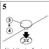
Attach Housing Caps to all Klix Cams by pushing neck of cap through center of cam.
