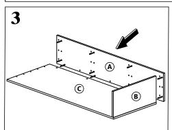
Attach Side Panel(B) to Back Panel(C) by using Cam Lock(1) and Klix Cam(2).
