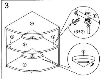
Insert Center Shelve Pins(E) into the pre drilled holes and place Adj. Shelve(5) at convenient distances.
