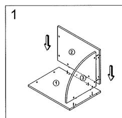
Attach the Side Panel-S (2) and Bottom Panel (3) to Side Panel-B (1) by using Cam Lock (A) and Klix Cam (B).
