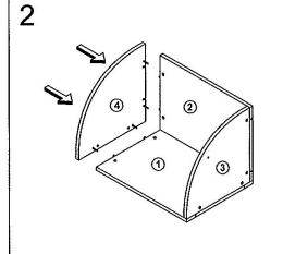
Attach Top Panel (4) to Side Panel (1 & 2) by using Cam Lock (A) and Klix Cam (B).
