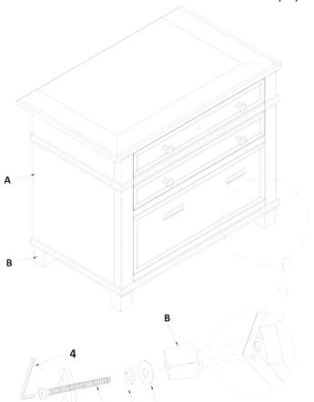
Turn the cabinet back ways, install foot (B) at each corner of the cabinet (A), locate dowels into aligning holes and secure in place using bolt (1) with spring washer (2) and flat washer (3).
