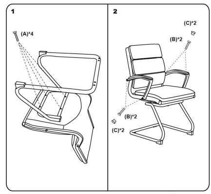
Insert and loosely tighten all screws. When assembly is completed, fully tighten all screws before using. This chair is only intended for sitting. Any other use will void the warranty.
