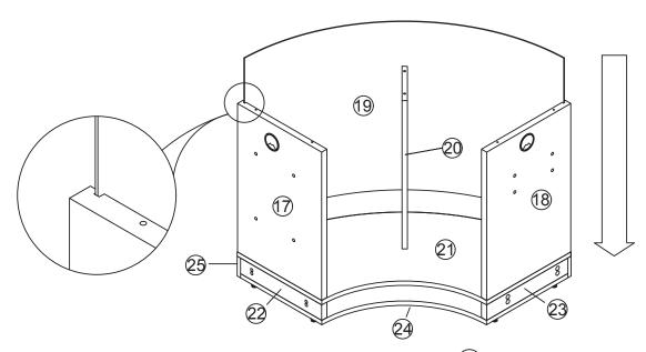
4. INSTALL "A" CAM SCREWS ON UNDERSIDE OF TOP 16. INSTALL "B" KLIX CAMS ON PANELS 17, 18 AND 20. CONNECT 16 TO 17, 18 AND 20 USING INSTALLED CAM SCREWS AND KLIX CAMS. TIGHTEN.
