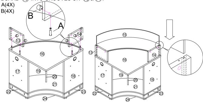
6. INSTALL "A" CAM SCREWS ON THE UNDERSIDE OF COUNTER TOP 12. INSTALL "B" KLIX CAMS ON SUPPORTS 13 AND 14. CONNECT 12 TO 13 AND 14. USING INSTALLED CAM SCREWS AND KLIX CAMS. TIGHTEN.
