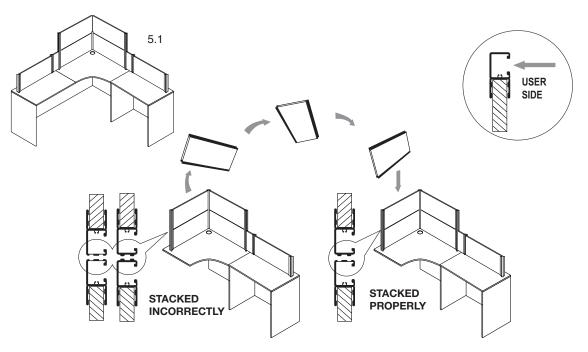
Please ensure panels are stacked properly - rails should fit in channels .
