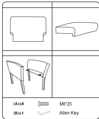
Insert and loosely tighten all screws. When assembly is completed, fully tighten all screws before using. This chair is only intended for sitting. Any other use will void the warranty.
