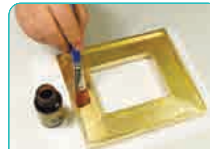
Step 4: Brush on sealer to protect the finish from possible abrasions in the future.
