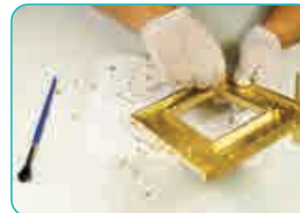
Step 3: Buff the surface of the frame to ensure adhesion.
