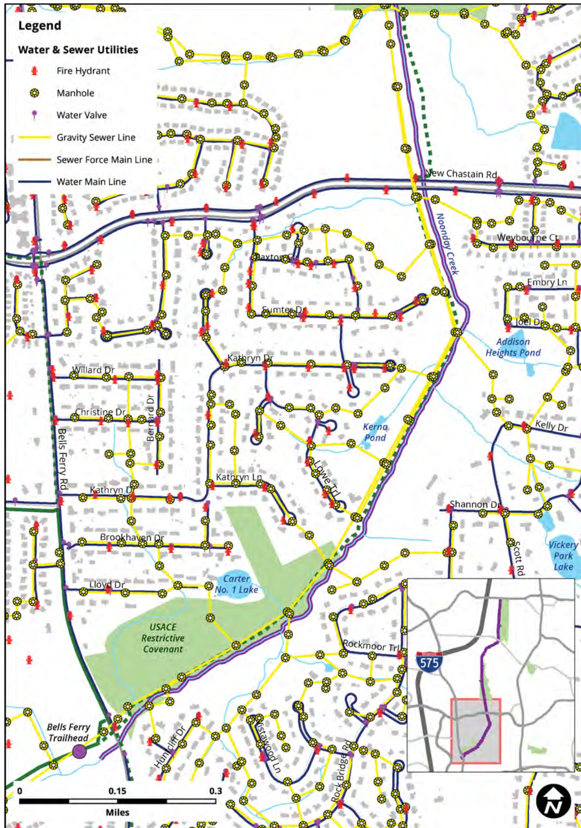
Figure 25: Water & Sewer Utilities Between Bells Ferry Road and Canterbury Greenspace
