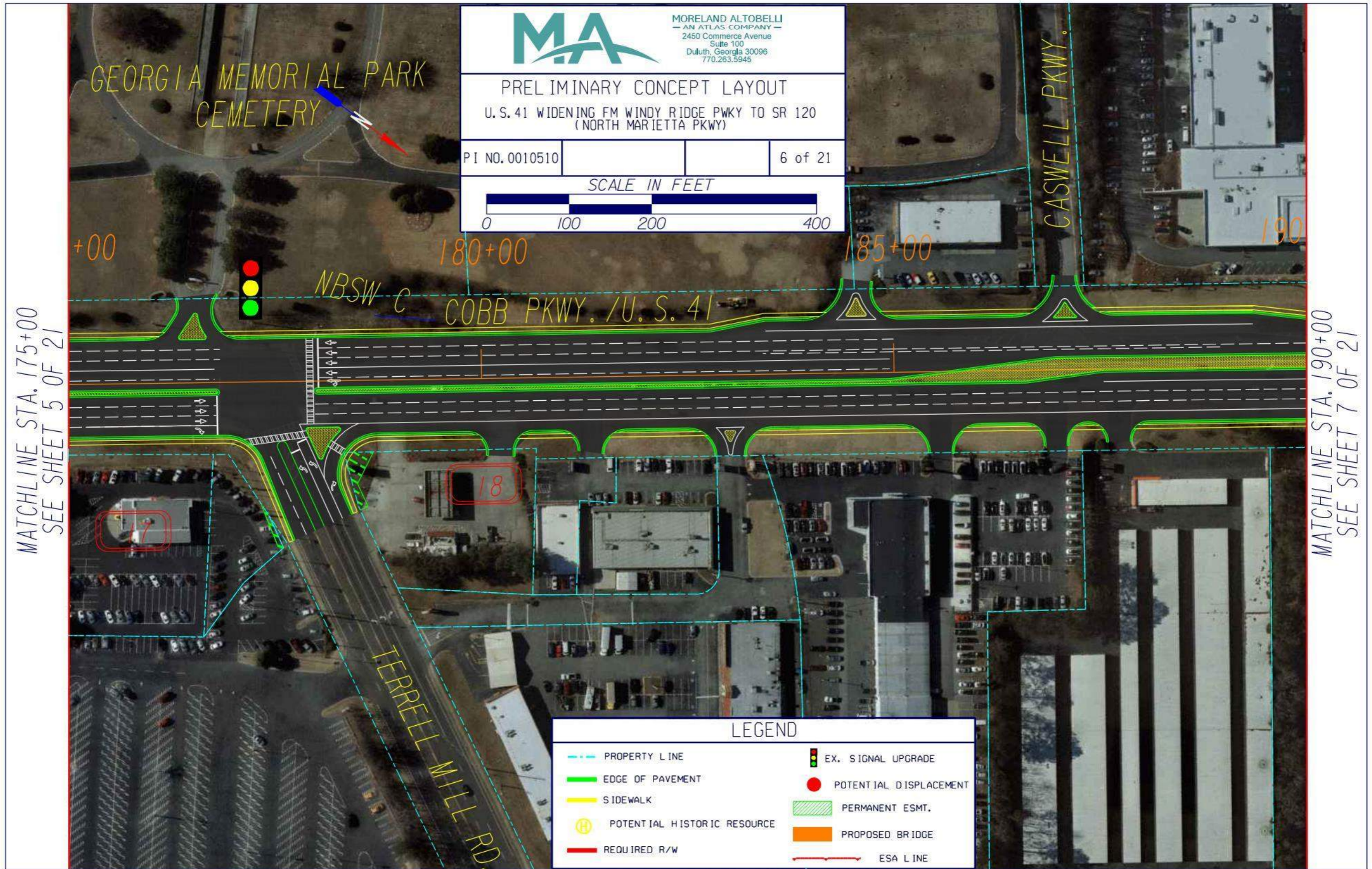
Figure 49: Prior Concept 2 – Continuous Flow Intersection (Sheet 3 of 3)
