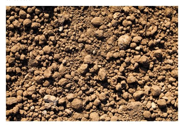
Soil for cob is generally easy to find in abundance and can generally be found all around the world. One good way to acquire the soil you need is to use what's excavated from your foundation trenches. You can also look at construction sites where this excavates soil is considered a 'waste product' and is hauled off to be dumped in a landfill. This costs them a lot of money and they might just be happy enough to deliver it to you for free!
