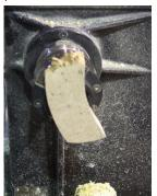
long axis. It was gripped with two jaws of the Talon chuck (two jaws had been removed). The top of the box was turned first. The completed box would be about  $\frac{3}{4}$ " thick. Mark turned a convex curve along the long axis of the box to produce a gentle, curved shape.
