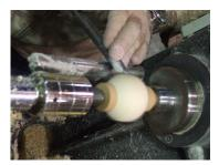
side of center. He turned each end of the cylinder to 5/8" diameter up to the one-inch lines. This made the length of the piece the same as its diameter. He used a detail gouge to remove waste at each end beginning sphere formation. Mark continued shaping using a one-inch Corian ring held against the surface as a guide to roundness. This completed the turning of the first of three axes (ak-sees) needed to complete the sphere. Then Mark removed the piece from
