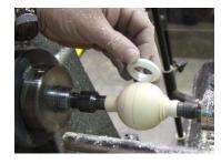
The same tools were used as before. This completed the male threads and the interior of the male portion of the box.
