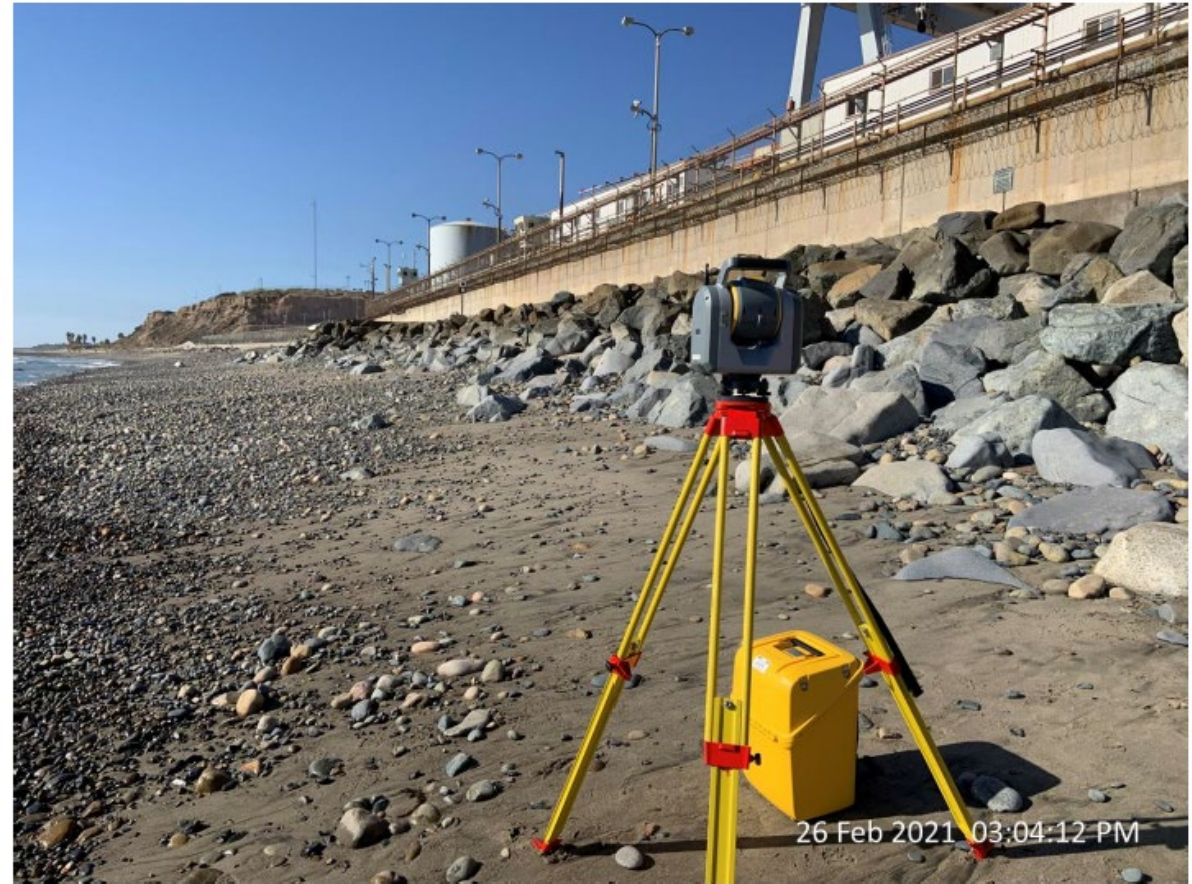
Figure 3-8. Trimble SX10 scanning total station.
