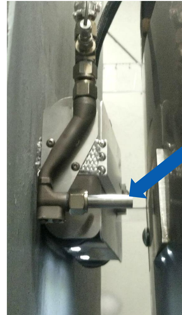
Cold spray nozzle attached to robot applying coating on canister mock-up at vendor facility
