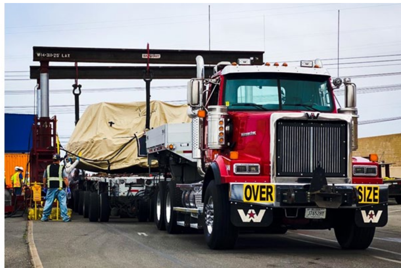
The team safely loaded and secured the Unit 2 reactor vessel head for shipment
