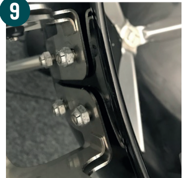
Here you can see the loose bolts: the hinge can easily be moved up and down along the slits for adjustment.
