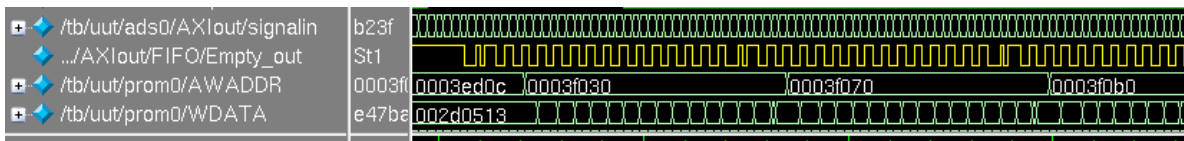
Figure 5.5: Modelsim showing the empty-signal, in yellow, being set high much of the time as data is written from the FIFO.
