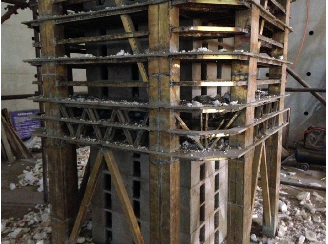
Detail of 1:30 model built for the seismic testing
