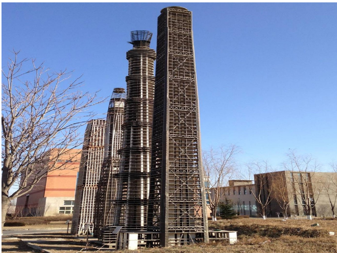
1:30 and 1:40 models of famous tall buildings tested on CBR's shake-test platform. The models are incredibly detailed and, despite the scaling factor, are some 40 ft (12 meters) in height.
