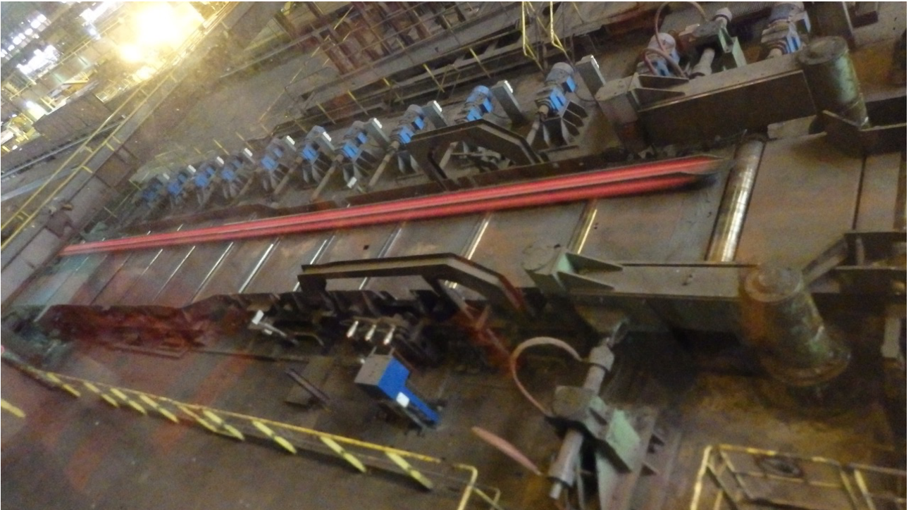
A red-hot beam is straightened after rolling.
