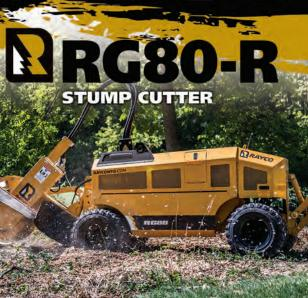
The RG80 has a powerful 85-HP (63-kW) Ford engine and a hydrostatic cutter wheel drive to let the operator vary cutter wheel rpm independent of engine speed. The propel system features Hi and Low travel speeds plus an integrated "creep mode" for precise handling while cutting. The RG80 has a wireless remote control that is sealed against dust, water, and other elements. The wide hydraulic backfill blade saves time during clean up and can easily be folded in for passing through gates.
