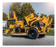
Fits onto a custom Rayco TRG trailer: The stump cutter is held to the trailer with simple and secure pins, eliminating chains and straps. The TRG trailer is equipped with TorFlex suspension and electric brakes.
