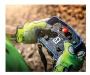
The wireless remote control unit is sealed against dust, water, and other elements.
