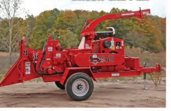
The ideal unit for residential tree services, utility line clearing, vegetation management, maintenance contractors and municipalities, this high-capacity chipper is now on a compact, economical design platform. The 8.2 lb., 6" (3.7 kg, 15.2 cm) channel frame rails increases structural strength while maintaining low unit weight.
